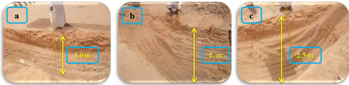
Fig. 3 Excavated trial pit
