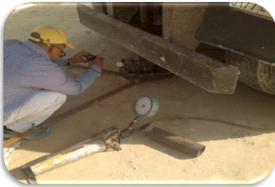
Fig. 21 Plate load test
