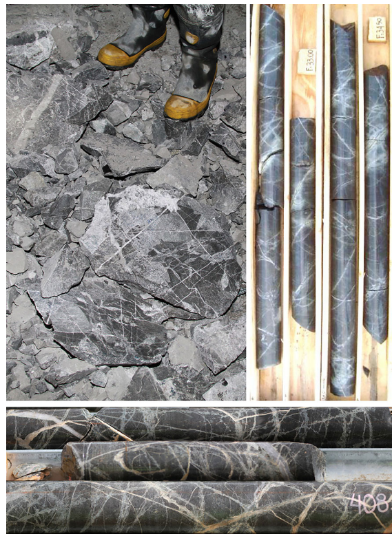
Fig. 1 Three examples of hydrothermal vein types of intrablock structures from Chile
