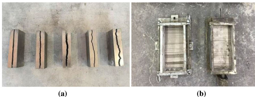
Fig. 1 Moulds for the joints of rock-like material. a Steel mould with Barton curve and b pouring mould
