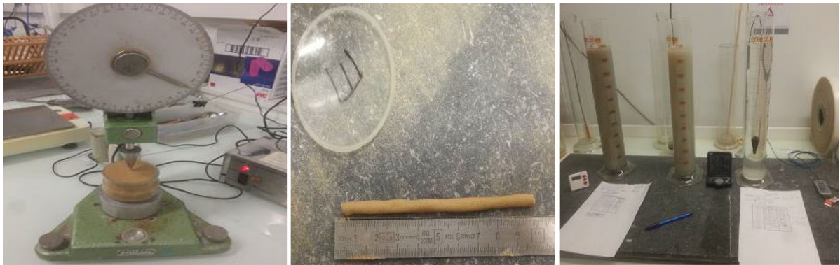
Fig. 15 Liquidity limits (WL), plasticity (Ip) and particle size analysis of the mixture
