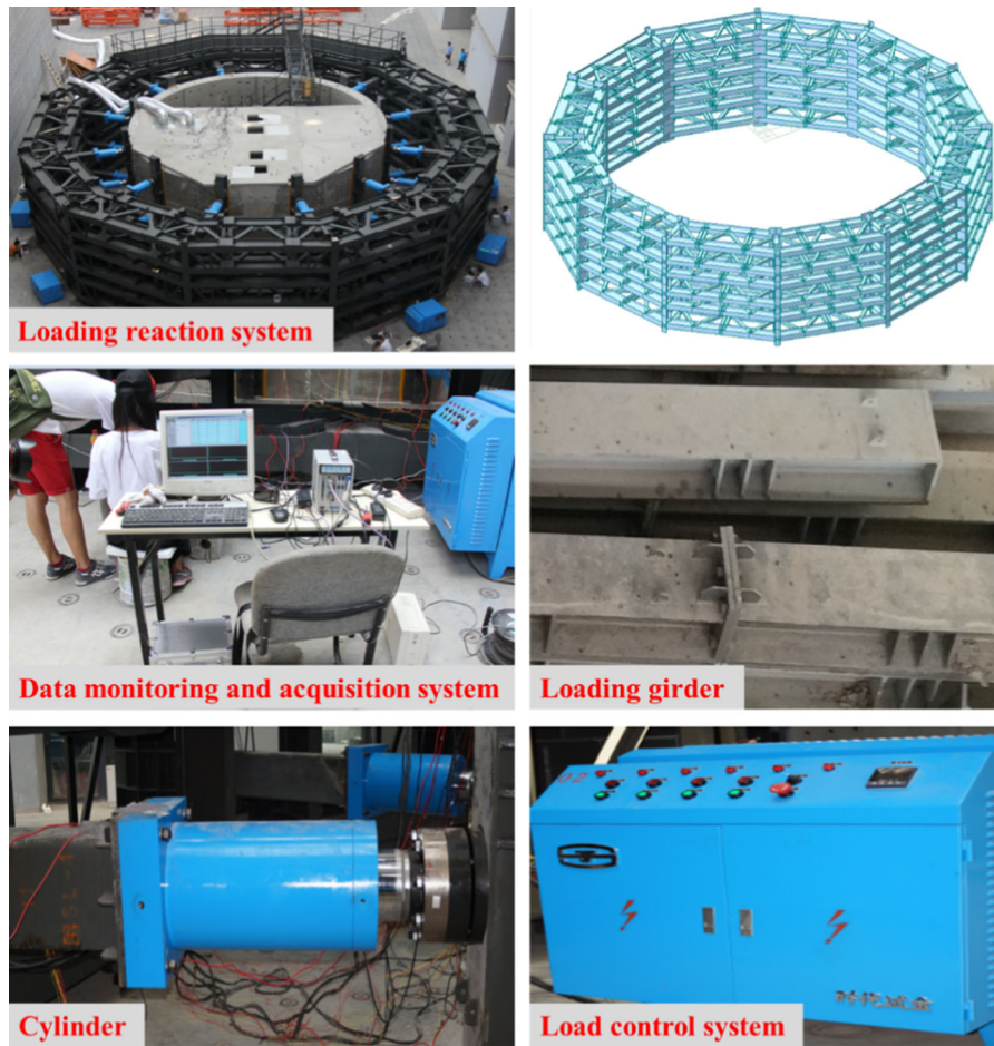
Fig. 2 Large mechanical test system for supporting structure of underground arch
