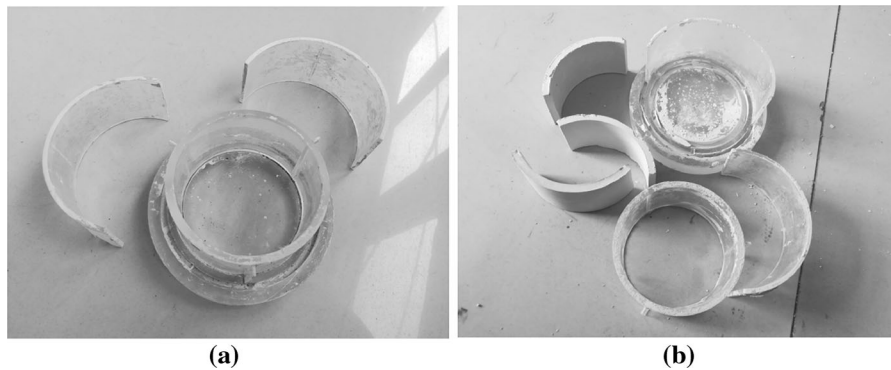
Fig. 4 Prefabrication of segmental lining. a Segmental lining mould; b Prefabricated lining segment
