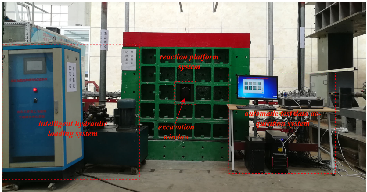
Fig. 2 Geo-mechanical model test device
