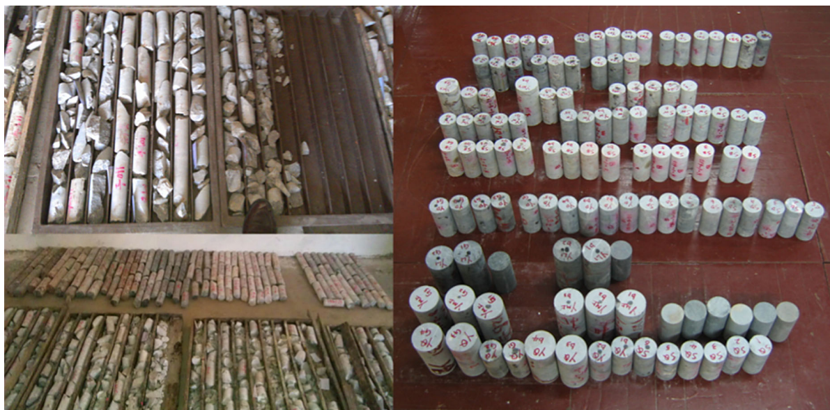
Fig. 5 Rock Samples taken from 1000 m depth; original samples (left) and prepared samples (right)
