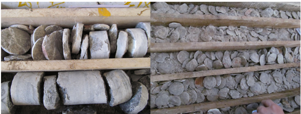
Fig. 2 Discs from drilled cores obtained from 1500 m depth
