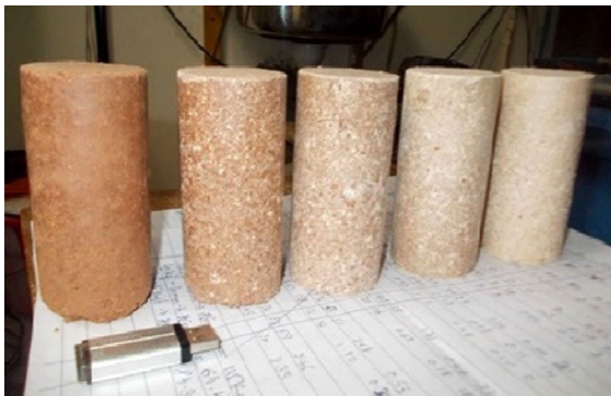
Fig. 2 Test specimens of various soil blends for cyclic tri-axial test
