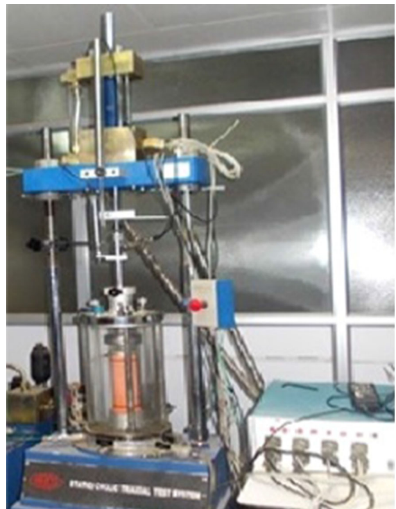
Fig. 3 The cyclic tri-axial test equipment
