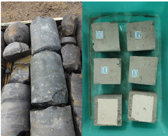
Fig. 5 Field drilling core and the specimen
