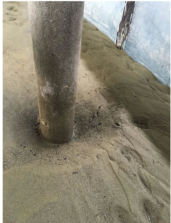
Fig. 5 Experimental run for circular obstruction
