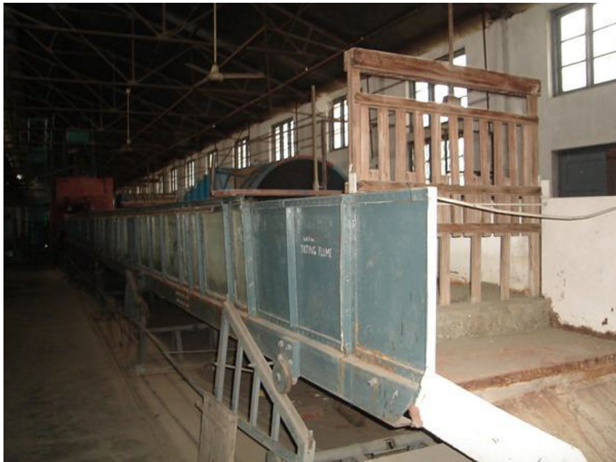
Fig. 1 Glass sided tilting flume used in the experimental study
