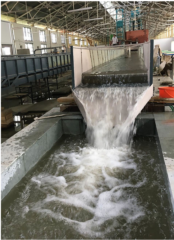
Fig. 4 Discharge measurement at the downstream using Sharp Crested Weir
