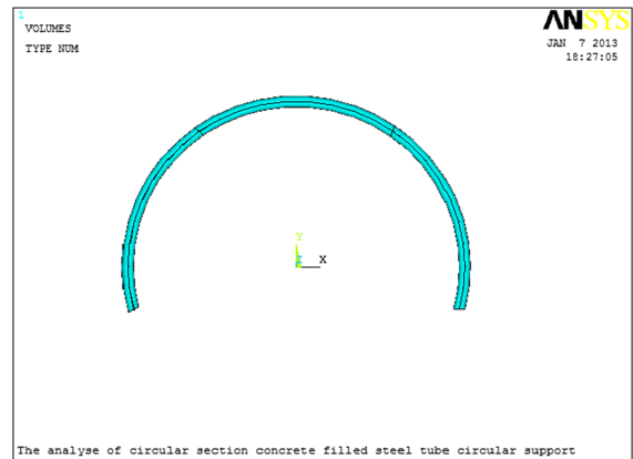
Fig. 10 Simplified model of CFSTS
