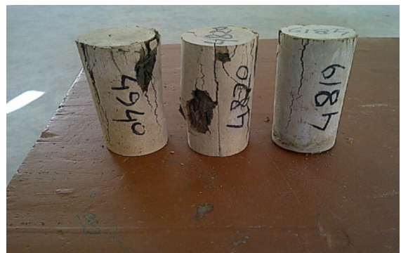
Fig. 3 Slag based stabilized soil sample after failure (30% slag content)
