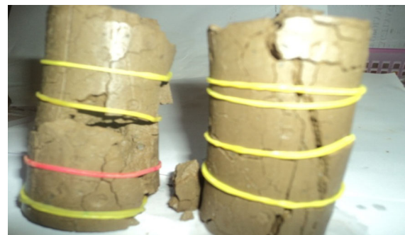
Fig. 13 Stabilized specimens after sodium sulphate exposure (cement stabilized)
