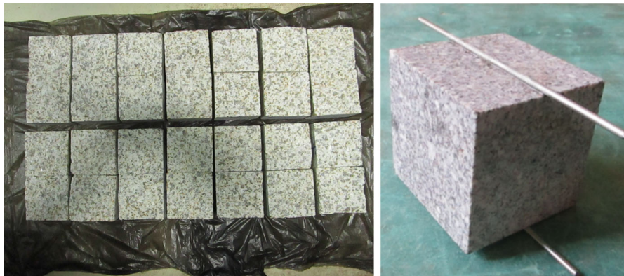
Fig. 1 Rock surfaces of Yellow Rust Granite obtained by the splitting testing
