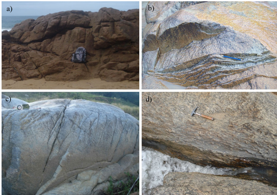
Fig. 2 a Scottsburgh outcrop with block structure, b White Mfolozi granitoid outcrop forming part of the basement rock, c Fafa granitoid exhibiting tension crack, d Fafa granitoid exhibiting a shear zone
