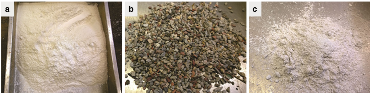
Fig. 2 Test material images a bentonite clay, b construction waste, and c GGBFS
