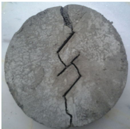
Fig. 6 Experimental results illustrating the breakage path of rock-like disc specimens containing three parallel cracks with constant spacing, S = 20 mm
