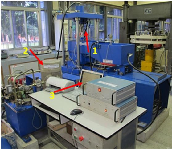
**Fig. 1** Photograph of large scale direct shear testing machine
