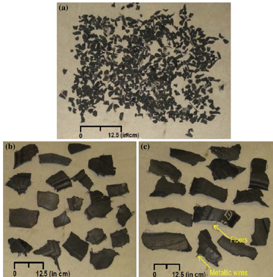
Fig. 2 Tire shred sizes considered in the study: a tire chips 9.5 mm in nominal size, b tire shreds 50-to-100 mm in length, and c tire shreds 100-to-200 mm in length
