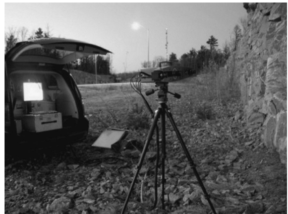
Fig. 8 3D stereo-topometric optical scanner utilized for the joint surface topography survey in the field (after Tatone and Grasselli 2009)
