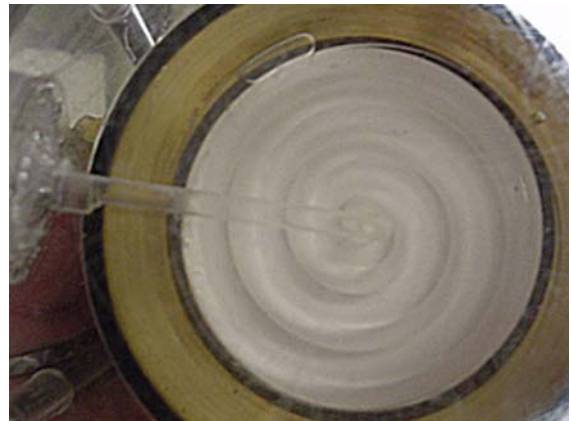
Fig. 14 Flushing diffused air from spiral groove of acrylic chamber
