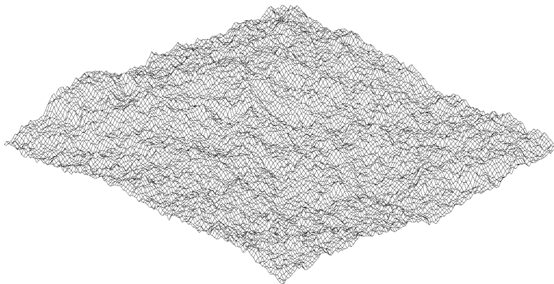
Figure 10. Generated fractional Brownian surface with fractal dimension equal to 2.5.
