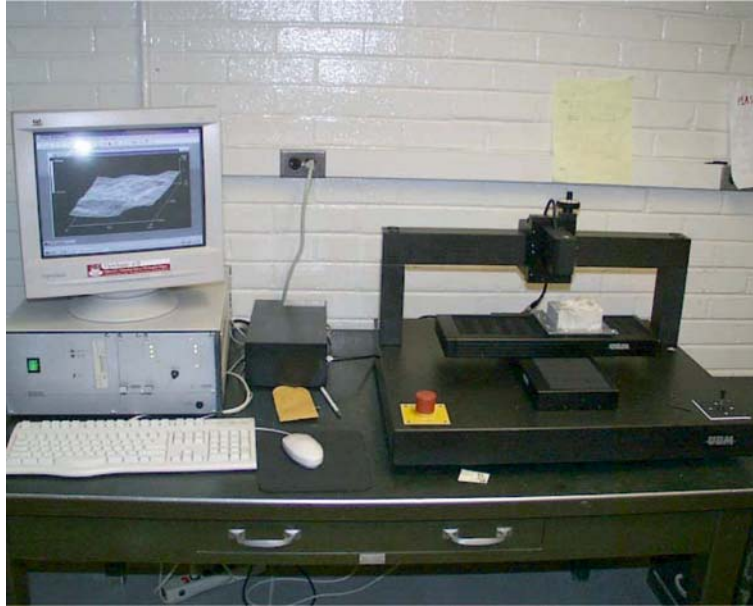
Figure 4. A photograph of the laser profilometer and data acquisition system.
