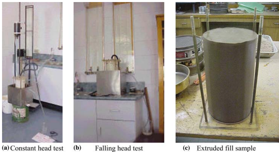
Figure 3. Permeability test set-up.
