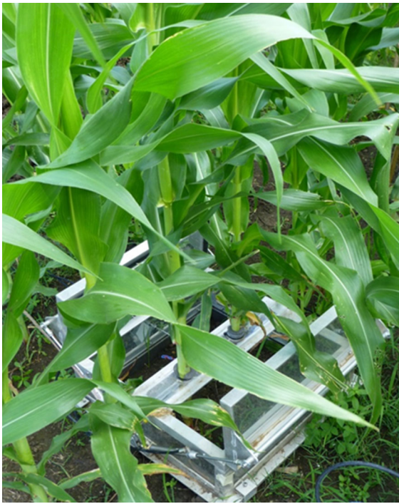
Fig. 2 Maize chamber used in the experimental set-up: maize stems are clamped airtight into a special chamber centerpiece with flexible sealing after the plants exceeded chamber height. Chamber base area is covering seeding row and interrow representatively
