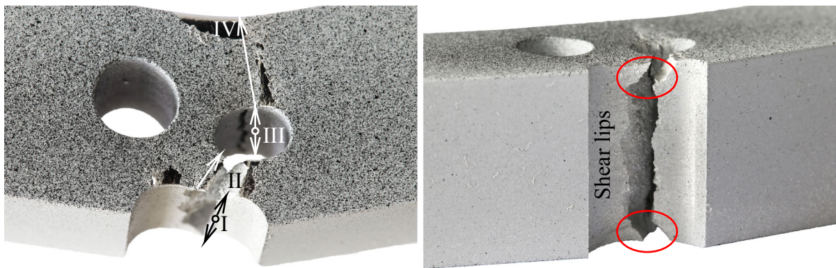
Fig. 19 Fractured specimen after the three-point bending test (Kubík et al. 2019)
