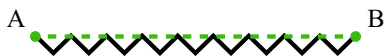
Fig. 4 Assuming rough surfaces orient at 45^\circ , microscopic surface roughness causes a path deviation of \eta = 1.41
