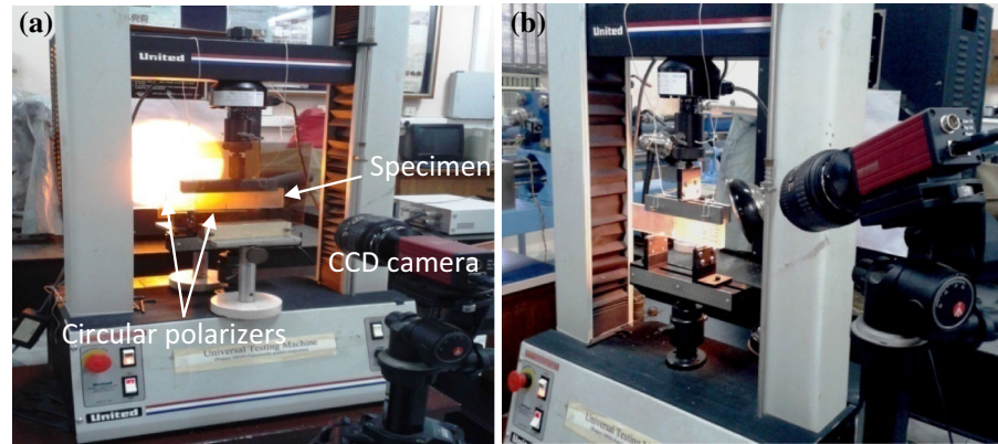
Fig. 2 Photographs of experimental setup for a photoelastic experiments, b observing crack growth
