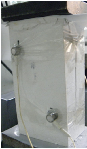
Fig. 7 Axial splitting failure of intact rock-like sample
