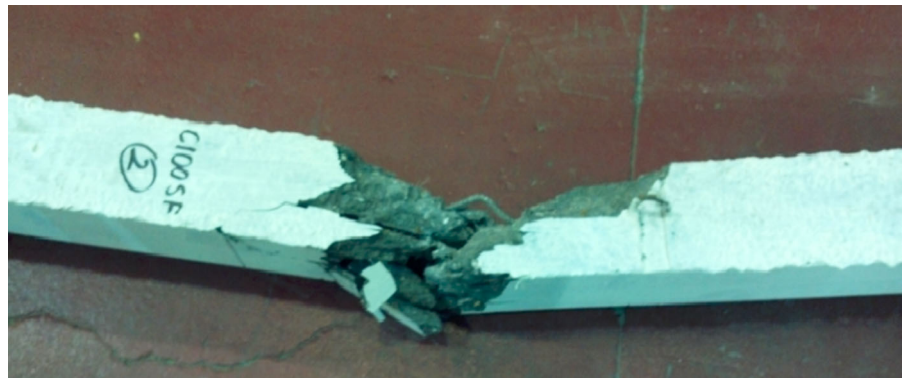
Fig. 26 Buckled C110+0.18% SF column 2
