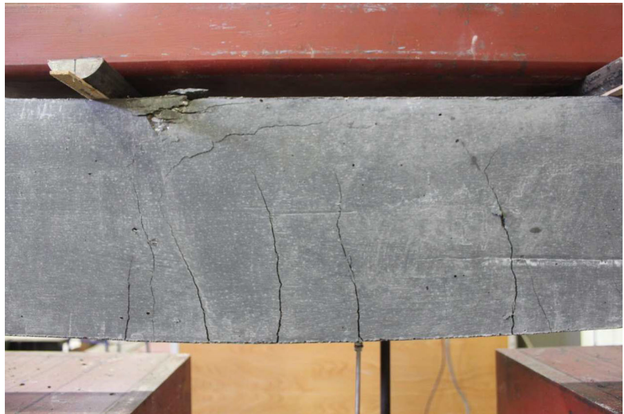
Fig. 9 Typical failure pattern of C100 + 0.2% SF beams of 225 mm depth
