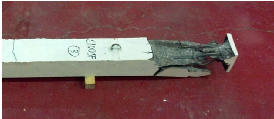
Fig. 27 Crushed C110+0.18% SF column 3
