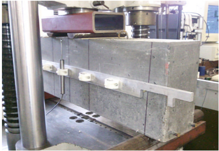
Fig. 17 Four point bending test set up of short beams over a span of 850 mm (span to depth ratio = 2.83)
