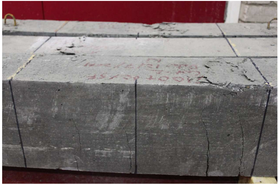
Fig. 10 Typical failure pattern of C100+0.2% SF beams of 200mm depth
