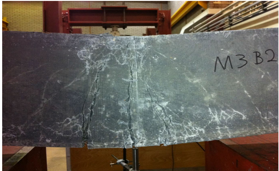
Fig. 15 A very high density of micro-cracks in a C85 + 0.75 % SF beam
