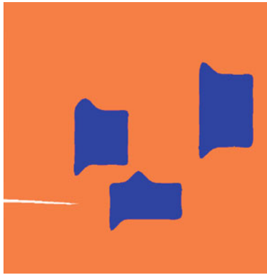
Fig. 5 Domain with three fibers and incipient crack at the beginning of the simulation, blue fiber material, red matrix material
