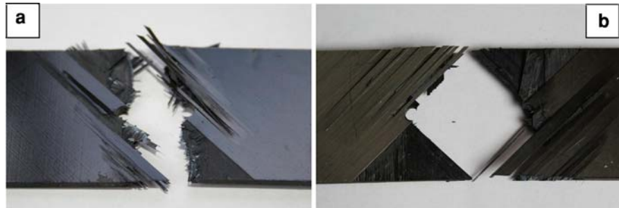
Fig. 15 Typical 2 mm thick failed specimens with w/d = 10 a sub-laminate level scaled b ply level scaled
