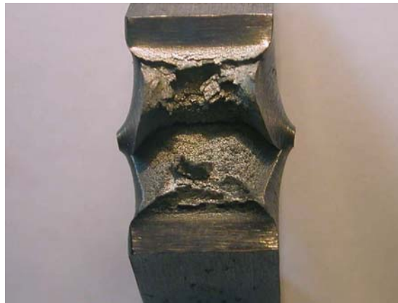
Figure 10. Test BM5; broken test sample, fracture surface 2.
