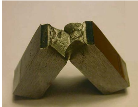
Figure 9. Test BM5; broken test sample, fracture surface 1.
