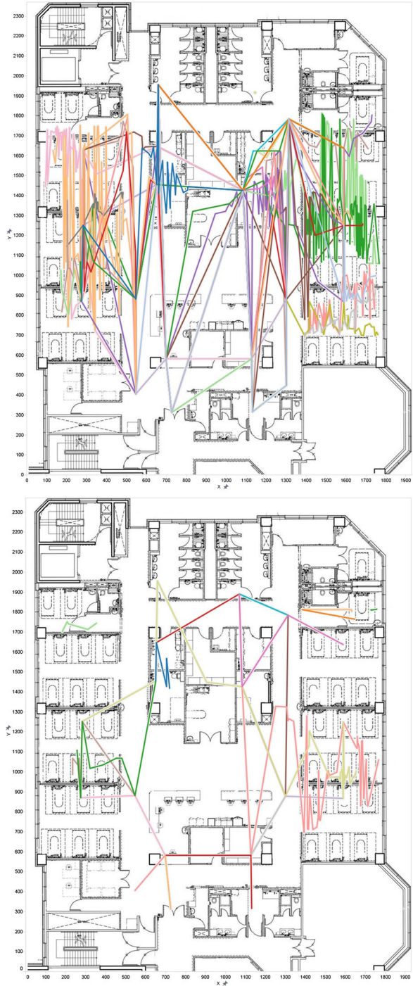
Fig. 9 Paths that the equipment moved for a selected day (at the top) and for a selected hour (at the bottom). The different colors represent different objects (Color figure online)
