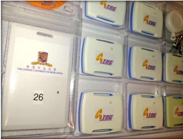
Fig. 4 The active RFID tags that were embedded in a plastic plate and the plates were placed on the medical equipment
