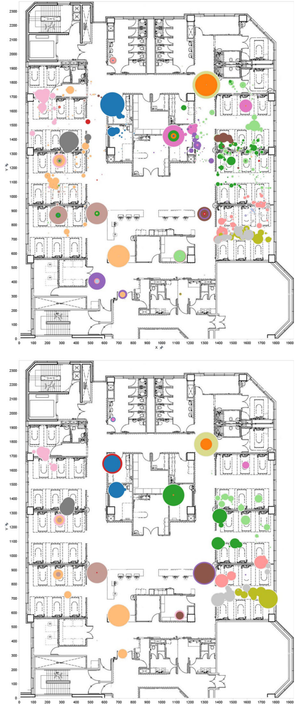
Fig. 8 Locations of the equipment for a selected day ( at the top ) and for a selected hour ( at the bottom ). The different colors represent different objects. The size of a circle is directly proportional to the total time that an equipment spent in the location (Color figure online)
