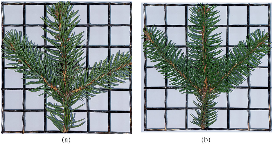
Figure 3. Specially designed sample holder with placed branches: (a) fir wood ( A. alba ); (b) spruce wood ( P. abies ).
