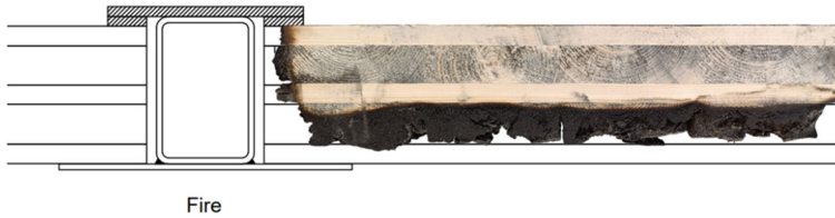
Figure 5. Residual cross-section of a CLT panel supported by an unprotected steel beam at 71 min of fire exposure. The CAD drawing corresponds to original dimensions.
