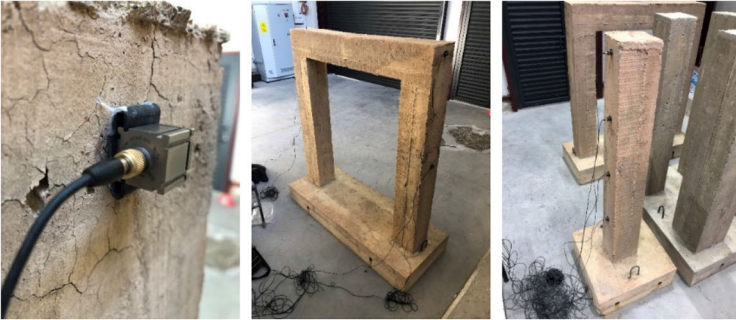
(b) Damaged concrete and RC models
