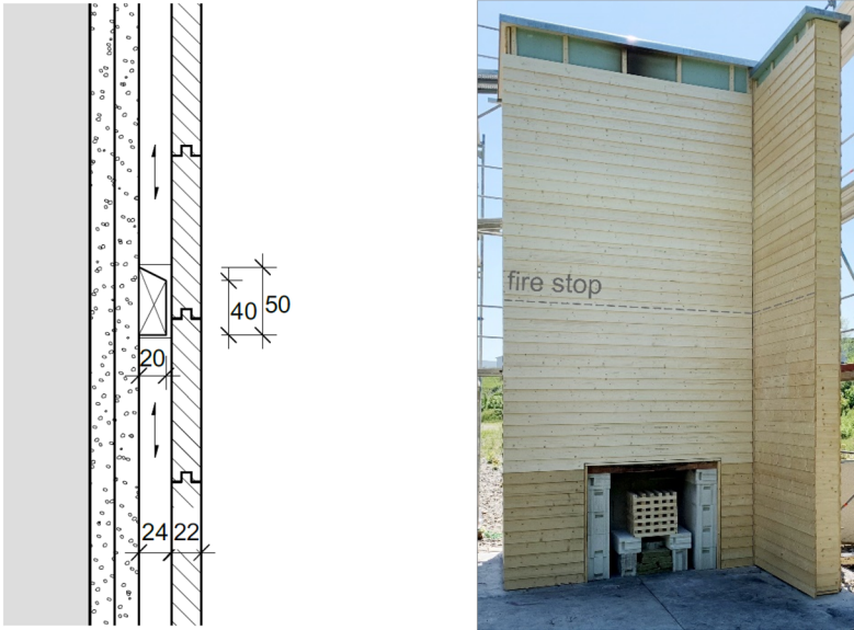
Figure 7. Vertical section and photo of the façade structure with visualized fire stop in Test 1 [in mm].
