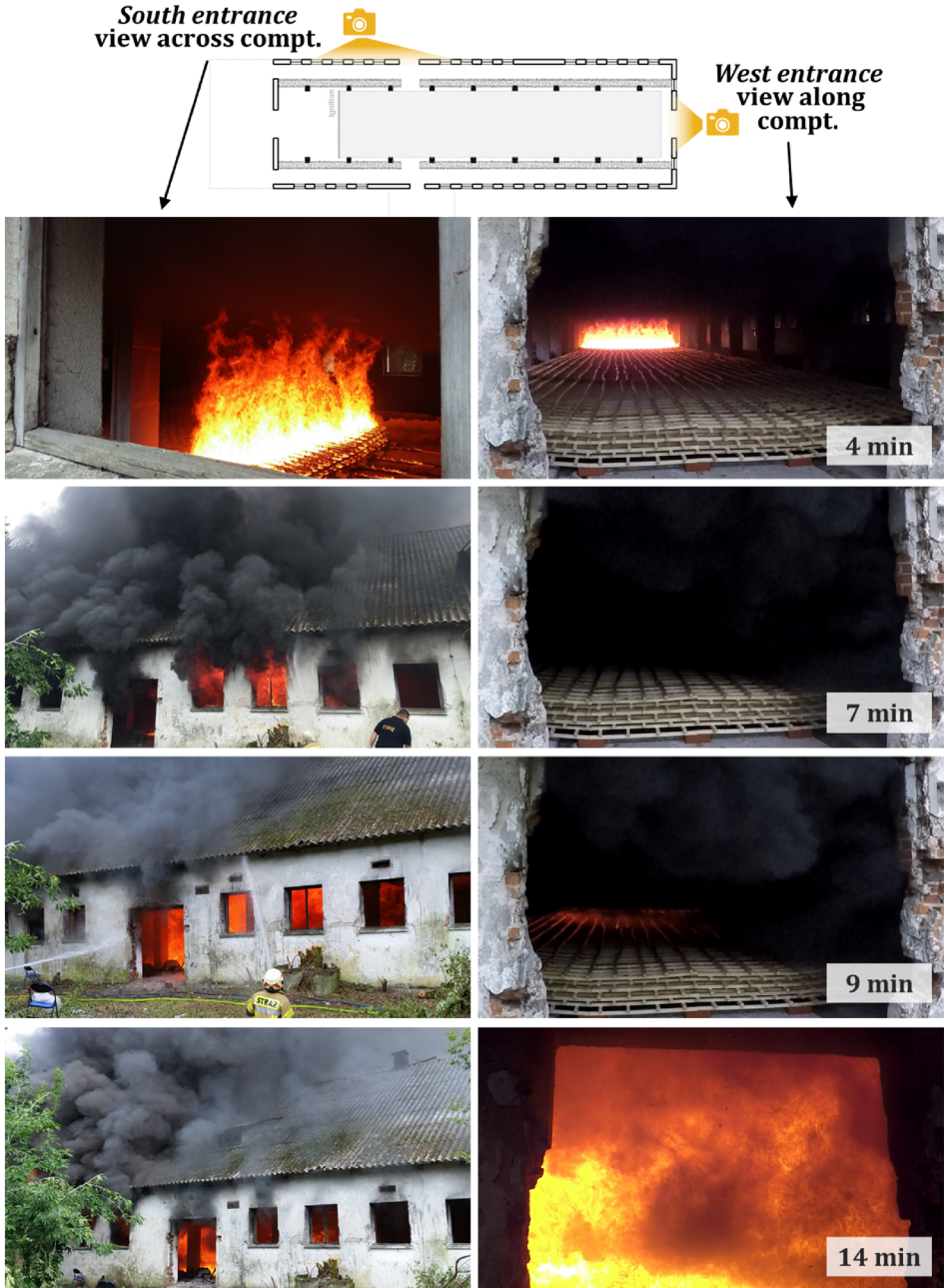
Figure 7. Photos taken from two different locations at four different times during the experiment showing fire development and progress. Left and right columns show view across the compartment taken outside of the South and West entrances, respectively.
