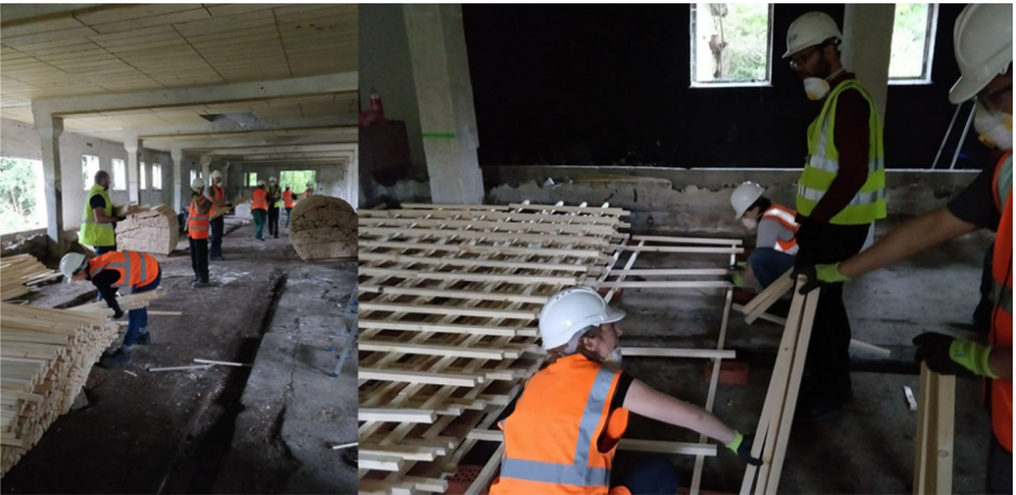
Figure 22. Illustration of the process of building the vast crib used to fuel the fire.
