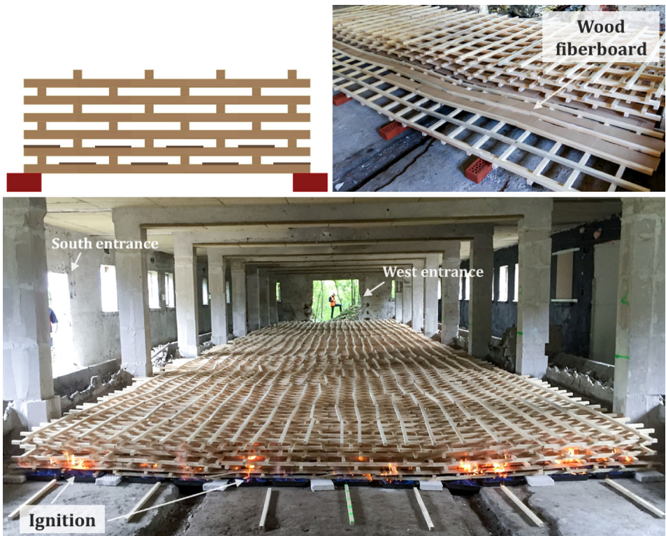
Figure 5. Illustration and photos of the final wood crib and fibreboard arrangement used as fuel for the x-ONE experiment. Wood stick dimensions were 3 cm × 3 cm × 1 m. The bottom image shows completed wood crib at the moment of ignition.
