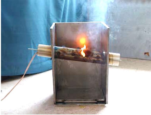
Figure 14. A droplet igniting on the hot manifold in the test rig of ISO 20823, from Deleanu et al. [62].
