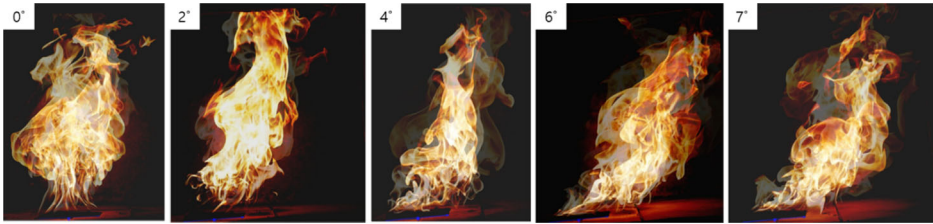
Figure 8. Images of tilted flame with respect to tunnel slope (images of intervals of 3 s are superimposed).
