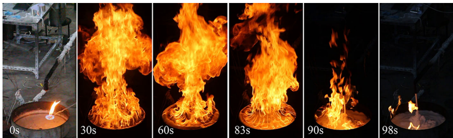
Figure 7. Typical process of the fire extinguishing test of firefighting foam.
