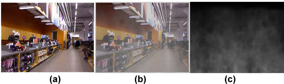
Fig. 4. An example of synthetic smoke image. A smoky image b can be served as the superposition of a clear background image a and a smoke layer image c.
