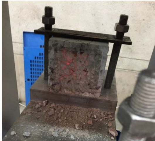
Figure 13. Direct shear tests setup- shear plane.
