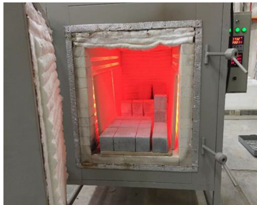
Figure 1. Electrical furnace and heating procedure.
