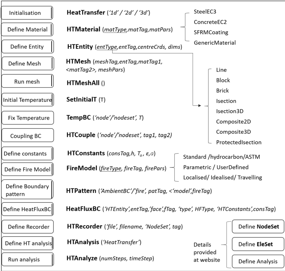
Figure 4. Definitions of commands for running thermal analyses in OpenSees.
