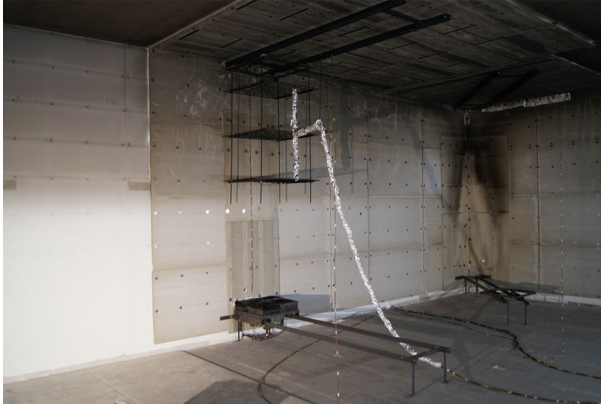
Fig. 2. Photograph of the compartment showing the position of the wall (left) and corner (right) burners. The three-dimensional array of thermocouples is seen above the wall burner.
