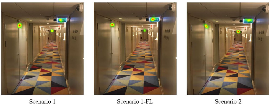
Figure 7. Schematic heat maps illustrating the number of fixations for each of the evacuation signs in the different scenarios. The colouring is relative with red meaning more fixations and green meaning less.
