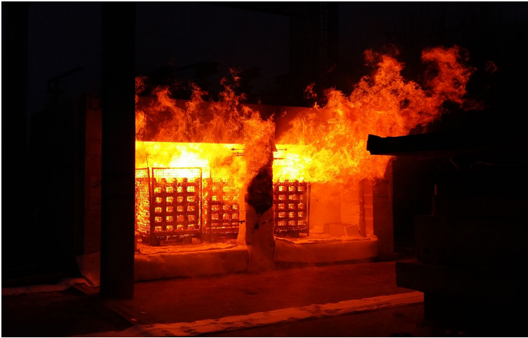
Figure 3. Compartment fire experiment with two openings and a low opening factor (Scenario 1).
