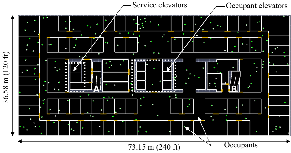
Figure 2. Typical floor layout with distribution of occupants. A, B: Required stairways as per IBC 2018 [6].
