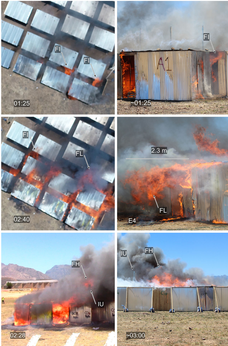
Figure 9. Photographic evidence documenting fire spread by direct flame impingement (FI), flame lengths out of dwelling vents (FL), and flame heights above roof level (FH), with 4 m tall instrument units (IU) pointed out for reference. Where times are not obtainable from the source footage, it is estimated based on correlation to other footage, and indicated as approximate (indicated with ~).
