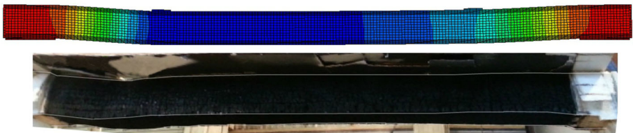
Figure 13. Comparison of failure modes in numerical model (above) and experimental beam (below) for C3 where a shear region failure between the support outside the furnace and the load application point can be seen [5].
