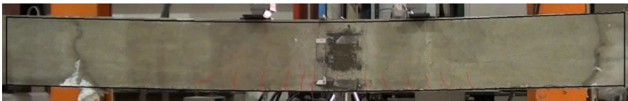
(b) Beam B4 at the beginning of residual tests
